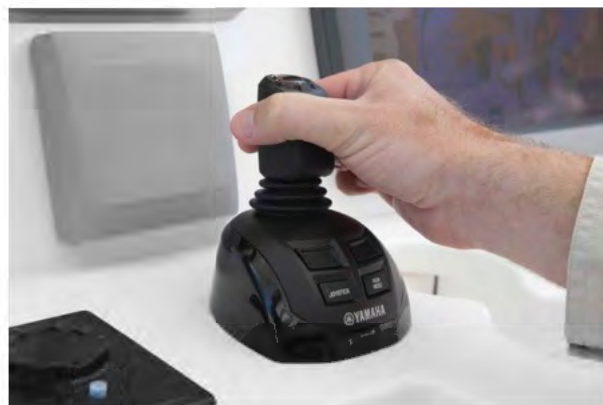
Yamaha's Helm Master lets you hold position and maintain orientation to the current and wind; Dockmate Twist is a wireless remote joystick device.
