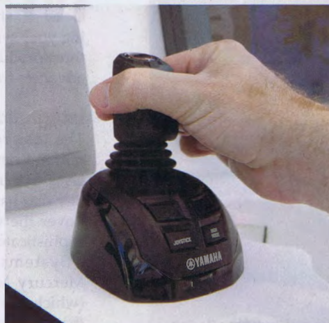
Yamaha's Helm Master (top and above left) lets you hold position and maintain orientation to the current and wind; Dockmate Twist is a wireless remote joystick device (above, right)
